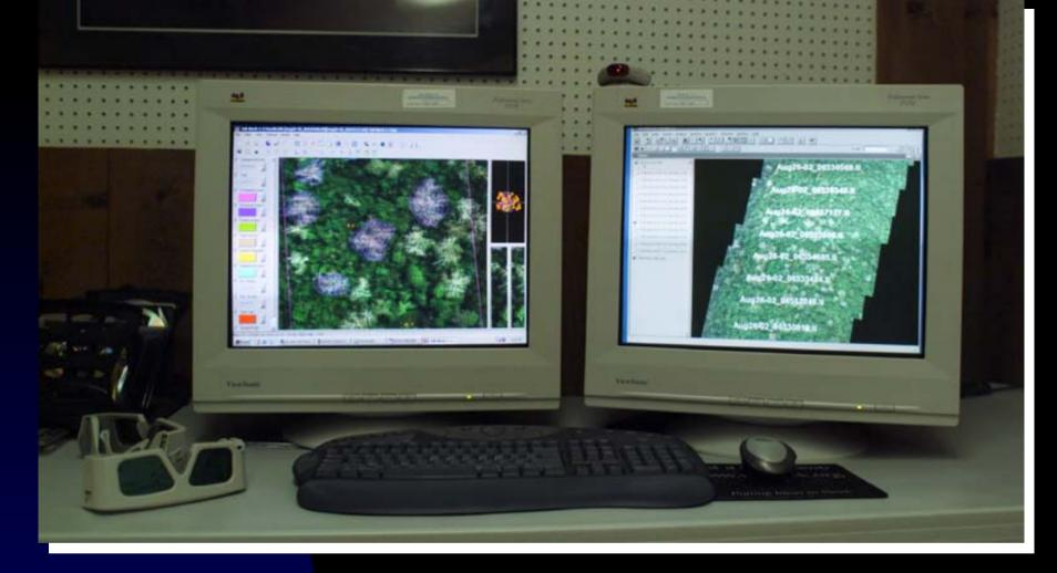
Dual monitor setup - ERDAS Stereo Analyst on one side, ArcView on the other. Polaroid glasses and IR transmitter provide the stereo effect on the monitor
